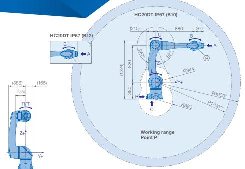
Absolute reach: S/L-Axis center of rotation to R/T-Axis center of rotation
