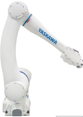
"Teach" and "Tool" buttons. These features offer time saving during the robot programming. The robot's arm geometry was designed to avoid pinch points (finger).
