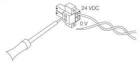
5. Connect the wires as shown in the following diagram.
