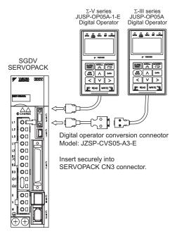
The digital operator can be connected or removed while the SERVOPACK power is ON.
