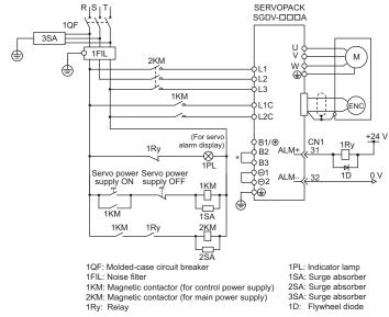
\* For the SGDV-R70A, -R90A, -1R6A, -2R8A, terminals B2 and B3 are not short-circuited. Do not short-circuit these terminals.
