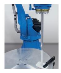
a TCP (Tool Center Point) can be set up very simply. Deviations and errors are thereby reduced. The handling and application doesn't require any further training or reading of a manual. The benefit is obvious or depends on the robot flange.
