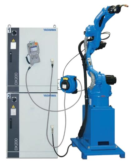
The automatic YASKAWA cable retraction system has been specially developed for the connecting cables of industrial robot teach pendants. This system is used to improve work safety in the production area and is a recognized accident prevention measure.
