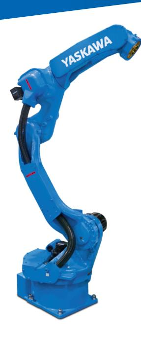
The MOTOMAN GP12 is a fast and precise 6-axis industrial robot with a payload capacity of up to 12 kg. With a reach of 1440 mm and a high repeatability of  $\pm$  0.02 mm, it is ideally suited to assembly tasks, but also universal handling tasks, CNC machine tool tending or packaging. Its streamlined modern industrial design minimizes the space requirements at the installation site.
