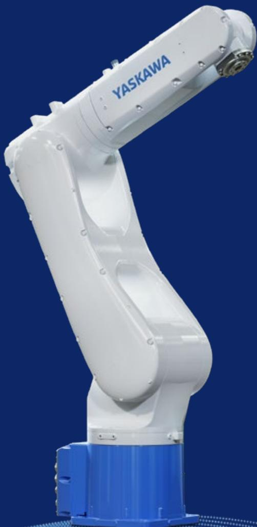
With a payload of 7 kg and a reach of 927 mm, the compact NEX7 manipulator is the right choice for a wide range of adaptive handling and assembly tasks. As part of the MOTOMAN NEXT platform, it is suitable for automation in which robots use sensors (e.g., cameras, force sensors) to detect, understand, evaluate, and autonomously respond to new situations and workpiece variants.
