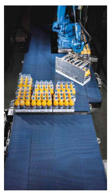
The bottle sorting table conveyor can be used either for free bottles, or bottles in multipack.
