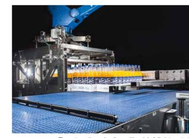
The automatic pusher for multipack is fully integrated in the MOTOMAN robot's control system.
