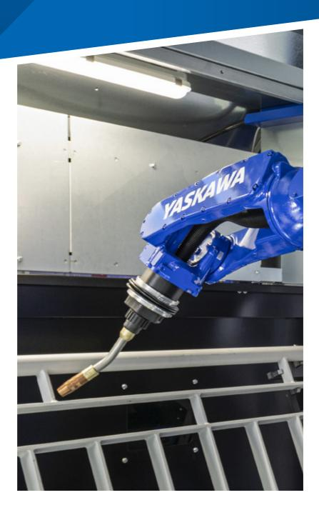
The Weld Length Check Function is a tool to control weld quality by checking the weld start point and weld length.
