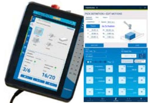
Designed to facilitate fast deployment of palletizing cells, the easy-to-use PalletBuilder extension app features an intuitive user interface that enables quick development and optimization of palletizing jobs. The included product database
