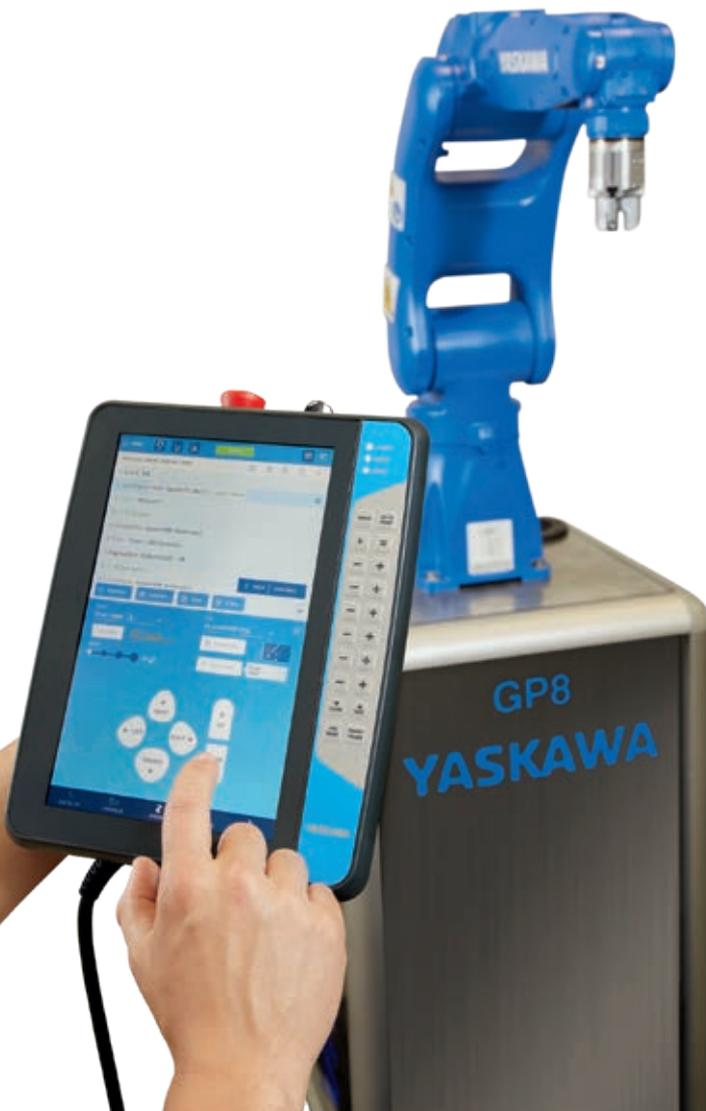
The Yaskawa Smart Pendant is an innovative teach pendant with a large 10-inch touch screen and offers a newly thought-out operator control concept.
