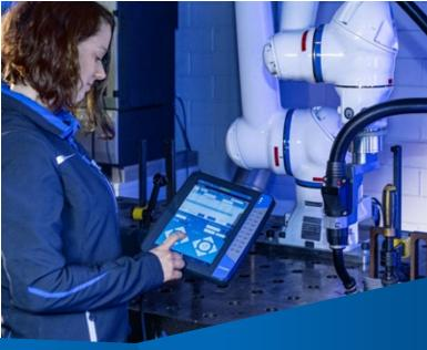
Use the Direct Teach buttons, Weld Builder or the Smart Pendant to program **Weld4Me CE**
