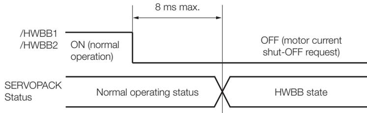
Note: 1. The OFF status is not recognized if the OFF interval of the /HWBB1 or /HWBB2 signal is 0.5 ms or shorter.
