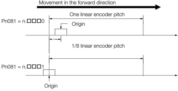
Observe the following precaution if you set Pn081 to n.□□□0 (Output phase-C pulses only in the forward direction).
