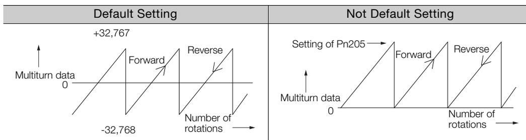
**Information** When the encoder is set to be used as a single-turn absolute encoder (Pn002 = n.□2□□), the multiturn data will always be zero. It is not necessary to reset the absolute encoder. Also, an alarm related to the absolute encoder (A.810 or A.820) will not occur.
