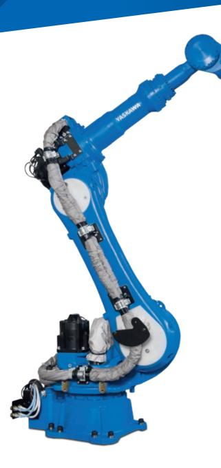
The MOTOMAN SP100 is a compact spot welding robot with 100 kg payload for servo-controlled lightweight welding guns. This technology allows very compact, cycle-time-optimized, energy-efficient and cost-effective welding cells to be installed in the smallest possible space. This robot is suitable for compact spot welding lines in car body construction with high robot density, for economical welding of small subassemblies, and for space-saving installation on a positioner.
