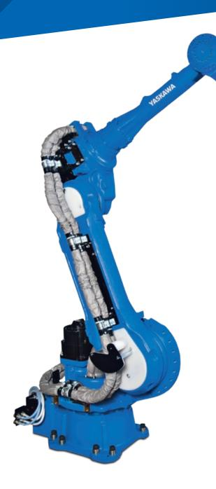
The MOTOMAN SP80 is a compact spot welding robot with 80 kg payload for servo-controlled lightweight welding guns. This technology allows very compact, cycle-time-optimized, energy-efficient and cost-effective welding cells to be installed in the smallest possible space. This robot is suitable for compact spot welding lines in car body construction with high robot density, for economical welding of small subassemblies, and for space-saving installation on a positioner.
