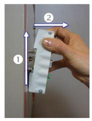
Push-up the B1 and pull it of the DIN rail.
