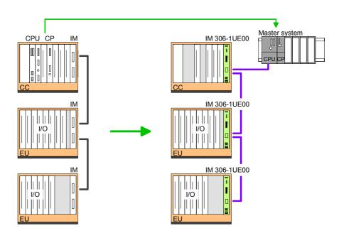
Deployment IM 306-1UZ00 IM 306-1UE00 (interrupt capability) If you want the support of modules with interrupt capability, this structure is to be used:
