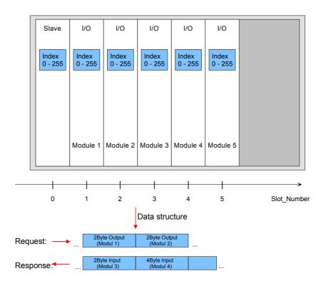
Each data block can be up to 244bytes. In the case of modular devices, the slot number is assigned to the modules. Compact devices are regarded as a unit of virtual modules. These can also be addressed whit slot number and index. Through the length specification in the read/write request, it is also possible to read/write parts of a data block.
