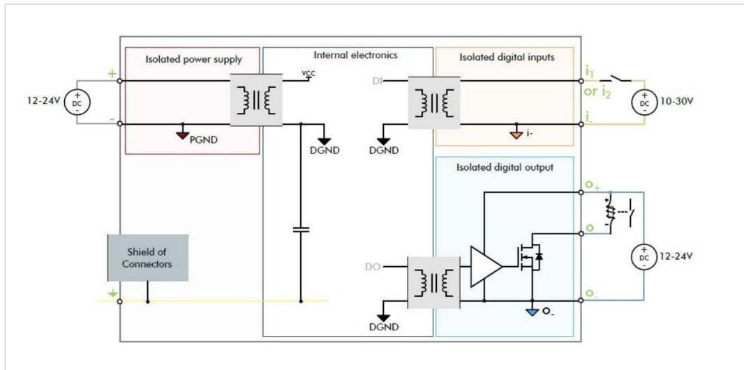
Fig. 18 Isolation Scheme for the Base Unit
