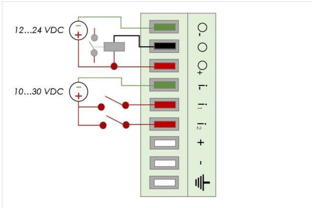
Fig. 16 Current scheme of the main connector
