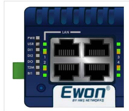
**Fig. 11** LED Panel of the Flexy 205
