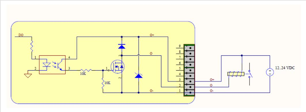
Fig. 17 External wiring for the Digital Output
