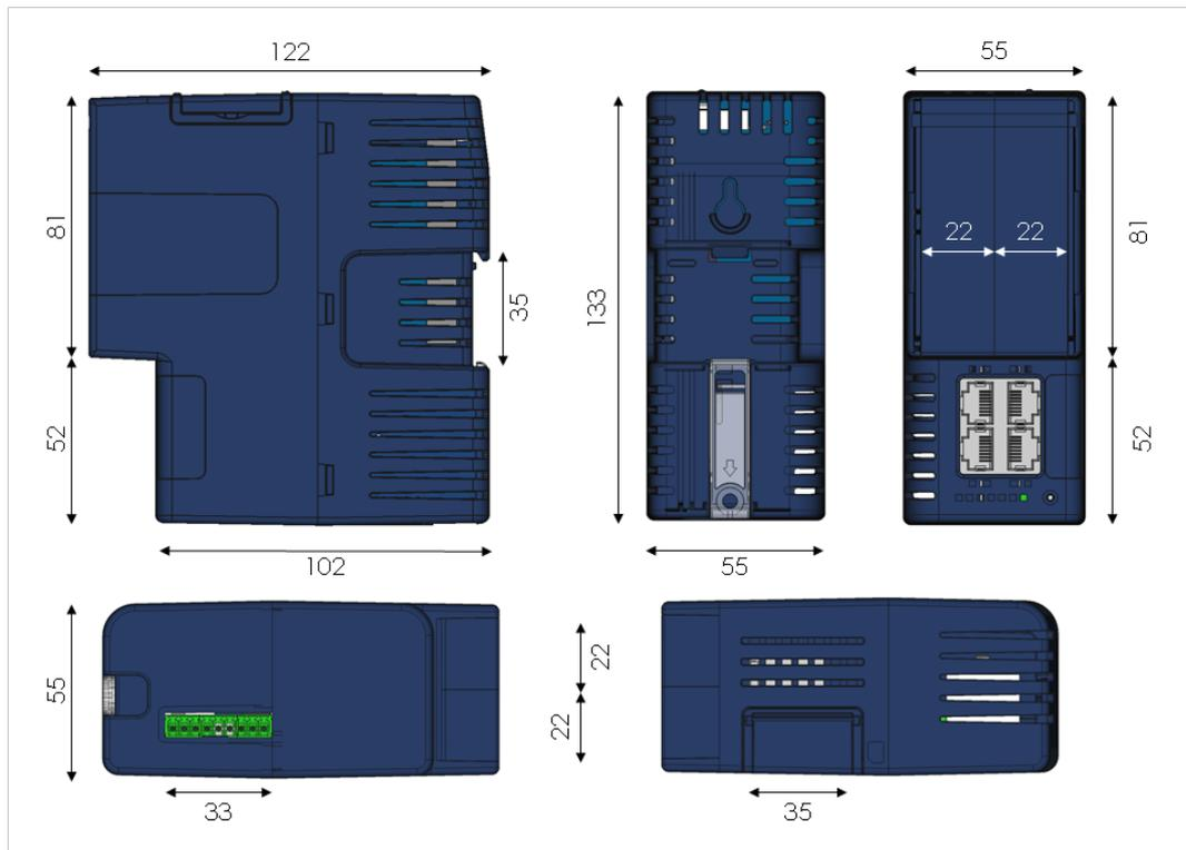
Fig. 7 Mechanical Dimensions
