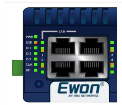
Fig. 9 LED Panel Example of a Flexy 205
