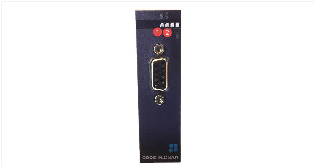
Fig. 3 Front Panel Leds
