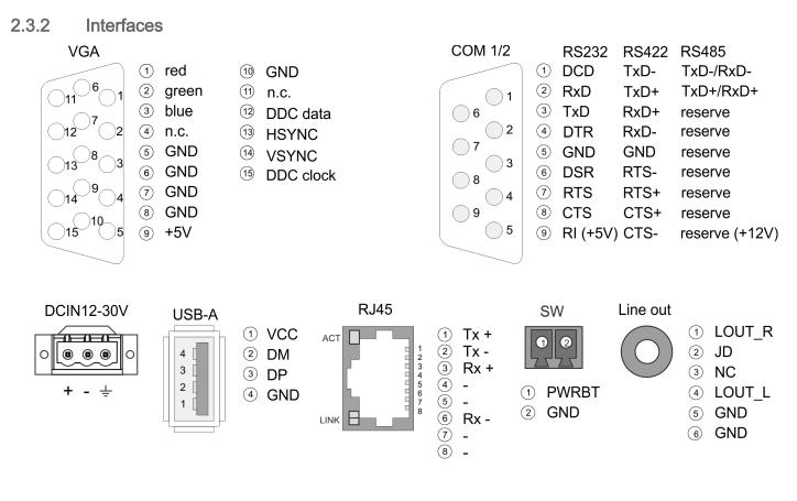
Power supplyThe Panel PC has got an integrated power supply. The power supply has to be provided<br/>with DC 12... 30V. For this you find an according DC 24V slot at the back. The power<br/>supply is protected against inverse polarity and overcurrent. The matching 3-pin plug<br/>connector is included in the scope of delivery.
