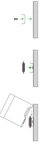
• Install the profile rail. Make sure that a clearance of at least 60mm exists above and 80mm below the middle of the profile rail.
