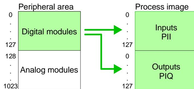
The process image is updated automatically when a cycle has been completed.
