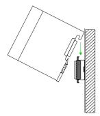
• Start at the outer left location with the installation of your header module and install the peripheral modules to the right of this.
