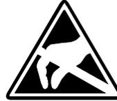
The symbol is located on the module, the module rack or on packing material and it indicates the presence of electrostatically sensitive equipment.
