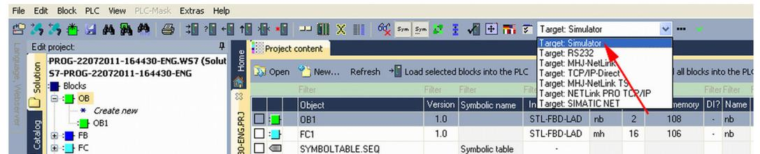
2. Transfer the blocks to the simulator with *[Load all blocks into the PLC]*.
