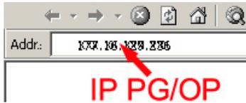
There is a web server, which can be accessed via the IP address of the Ethernet PG/OP channel with an Internet browser. At the web page information about the CPU and its connected modules can be found. [Chap. 5.6 'Hardware configuration - Ethernet PG/OP channel' page 39](#)
