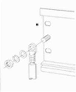
1. Bolt the profile rail with the background (screw size: M6), so that you still have minimum 65mm space above and 40mm below the profile rail.
