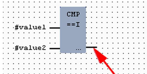
2. ➤ Open in the *catalog* the category '*Bit logic*' and select the function '*--[=]*'. The inserting of '*--[=]*' corresponds to the WinPLC7 shortcut *[F7]*.
