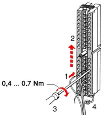
6. ➤ Put the included cable binder around the cable bundle and the front connector.
