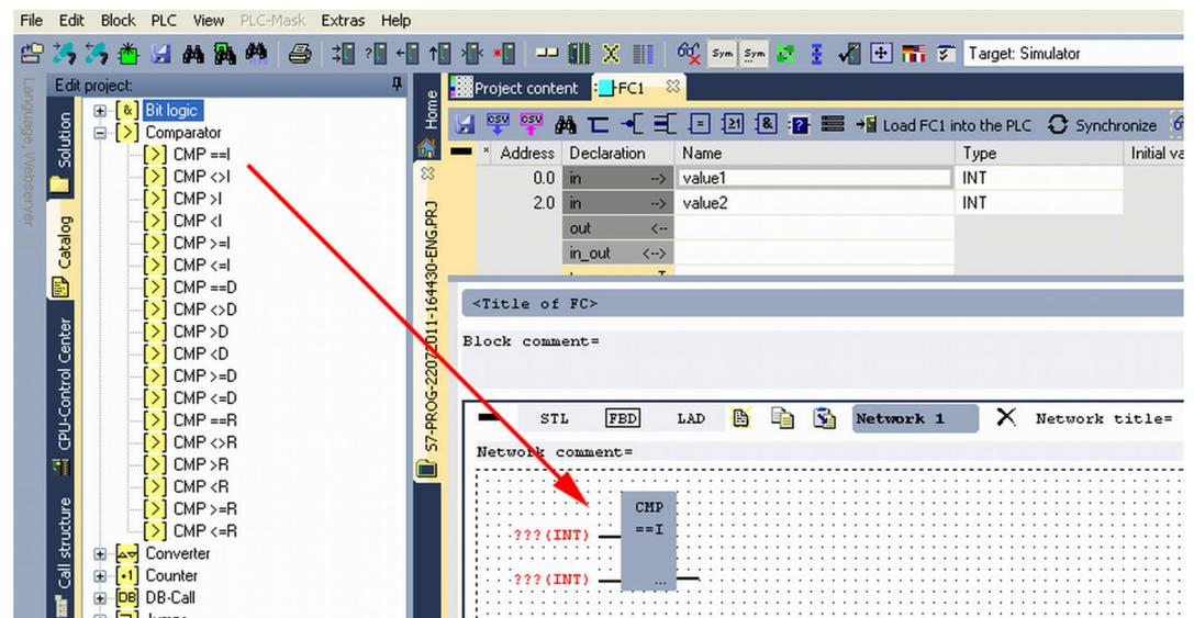
4. Click to the input left above and insert *value1*. Since these are block parameters a selection list of block parameters may be viewed by entering "#".
