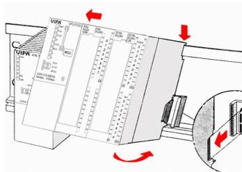
5. Stick the power supply to the profile rail and pull it to the left side to the grounding bolt of the profile rail.
