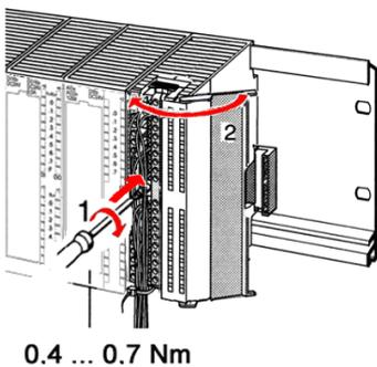
8. ➤ Bolt the fixing screw of the front connector.
