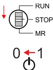
1. Switch the operating mode switch of your CPU in position STOP.
