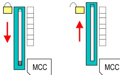
To remove, slide the sliding mechanism up again and push the storage media against the spring pressure until it is unlocked with a click.
