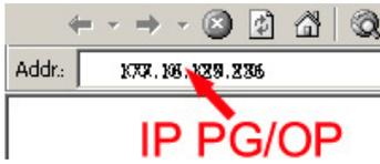
There is a web server, which can be accessed via the IP address of the Ethernet PG/OP channel with an Internet browser. At the web page information about the CPU and its connected modules can be found. [Chap. 5.7 'Hardware configuration - Ethernet PG/OP channel' page 54](#)
