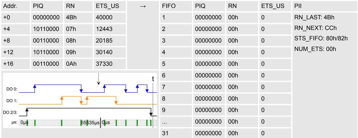
**i** Please consider the ETS modules can only effectively be used together with head modules, which have an integrated µs ticker. The Ethernet coupler with ModbusTCP 053-1MT00 for example does not have an µs ticker.
