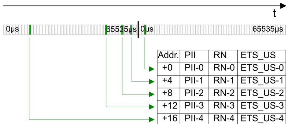
**Input area** The input range is used for status message. At CPU, PROFIBUS and PROFINET the input respectively output area is embedded to the corresponding address area.
