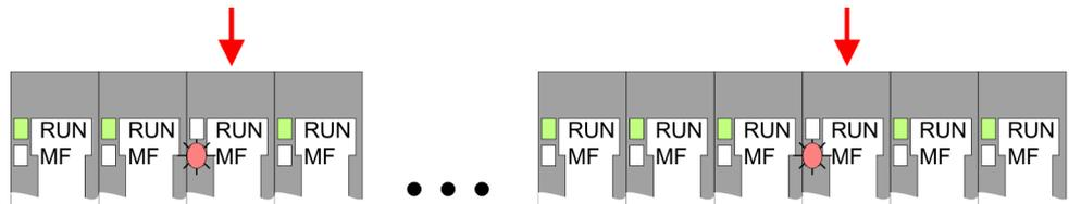
**Behaviour:** After PowerON the MF LED of one module respectively more modules flashes. The RUN LED remains off.
