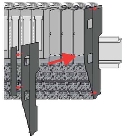
7. After mounting the whole system, to protect the backplane bus connectors at the last module you have to mount the bus cover, now. If the last module is a clamp module, for adaptation the upper part of the bus cover is to be removed.
