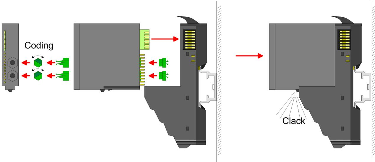
Each electronic module has on its back 2 coding sockets for coding jacks. Due to the characteristics, with the coding jack 6 different positions can be plugged, each. Thus there are 36 possible combinations for coding with the use of both coding sockets.
