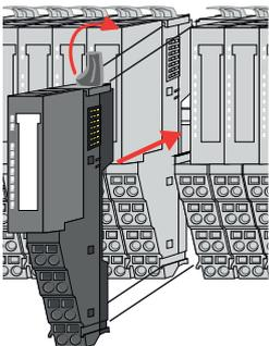
7. ➤ To mount the module put it to the gap between the both modules and push it, guided by the stripes at both sides, to the mounting rail.
