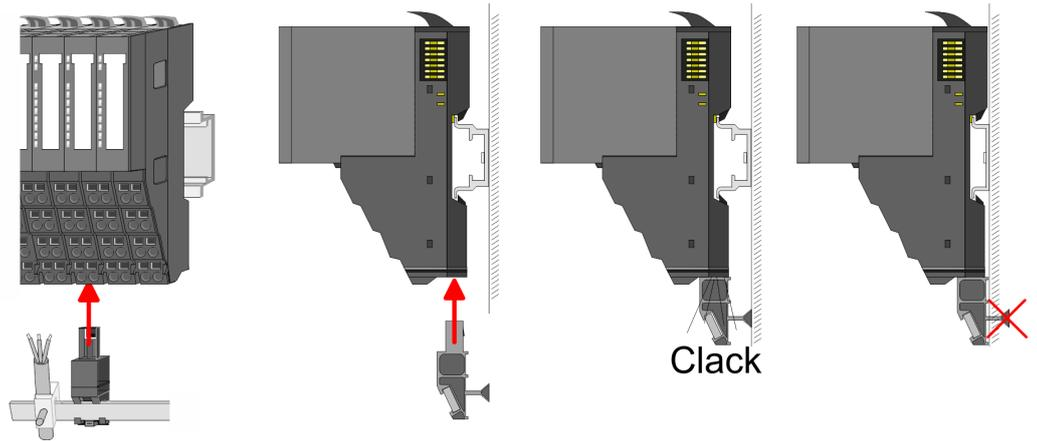
3. Attach the cables with the accordingly stripped cable screen and fix it by the shield clamp with the shield bus.
