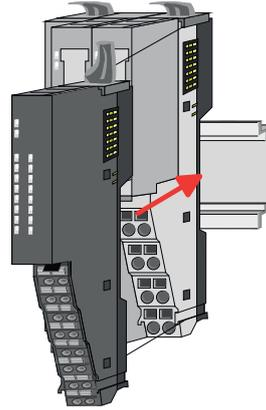
4. For mounting turn the locking lever of the module upwards until it engages.
