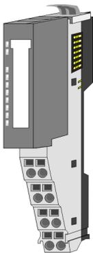
In the System SLIO the power supply is established by power modules. These are either integrated to the head module or may be installed between the periphery modules. Depending on the power module isolated areas of the DC 24V power section supply may be defined respectively the electronic power supply may be extended with 2A. For better recognition the colour of the power modules are contrasting to the periphery modules.
