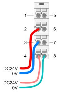
For wires with a core cross-section of 0.08mm<sup>2</sup> up to 1.5mm<sup>2</sup>.
