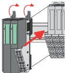
**<u>4.</u>** Turn all the locking lever of the bus coupler to be exchanged upwards.
