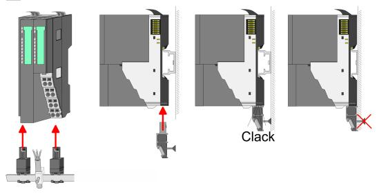
**3.** Attach the cables with the accordingly stripped cable screen and fix it by the shield clamp with the shield bus.
