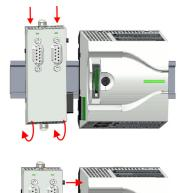
**3.** To mount plug the extension module from the top onto the mounting rail and turn the extension module downward until it rests on the mounting rail.
