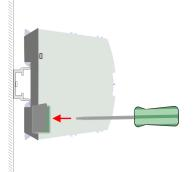
**2.** The extension module has a locking lever on the upper and lower side. Pull these levers outwards as shown in the figure, until these engage audible.
