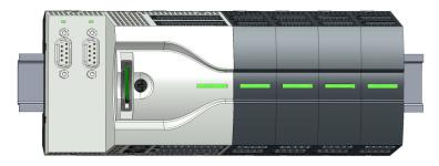
The System MICRO is a modular automation system for assembly on a 35mm mounting rail. By means of periphery modules this system may be adapted matching to your automation tasks. In addition, it is possible to expand your CPU by appropriate interfaces. The wiring complexity is low, because the DC 24V electronic section supply is integrated to the backplane bus and this allows replacement with standing wire.
