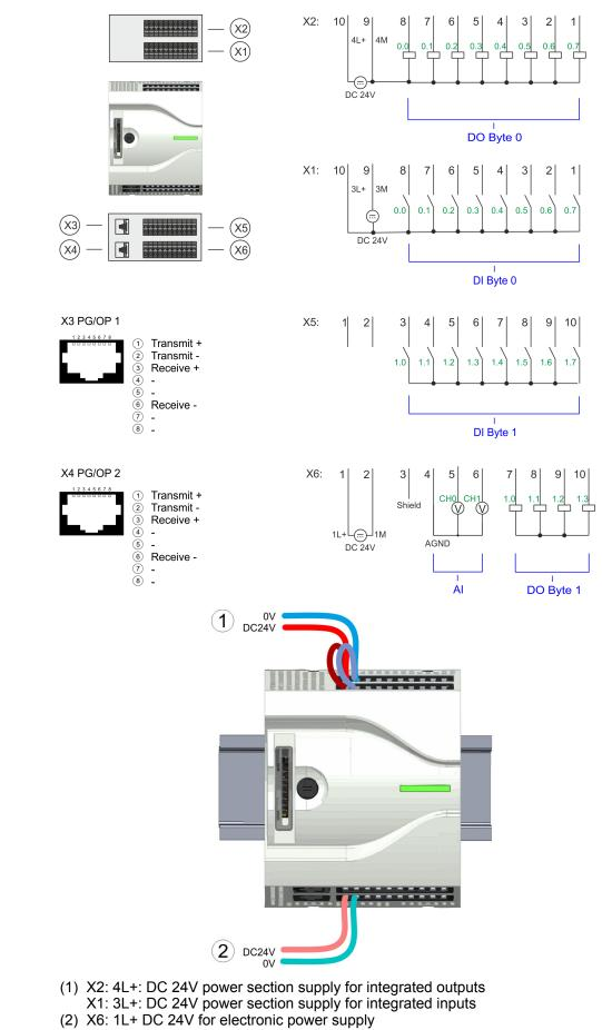
Wiring > Wiring CPU
