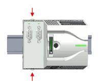
**5.** To fix the extension module at the mounting rail, move the locking levers back to the initial position.
