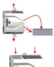
3. Pull the locking levers of the CPU outwards until these engage audible.
