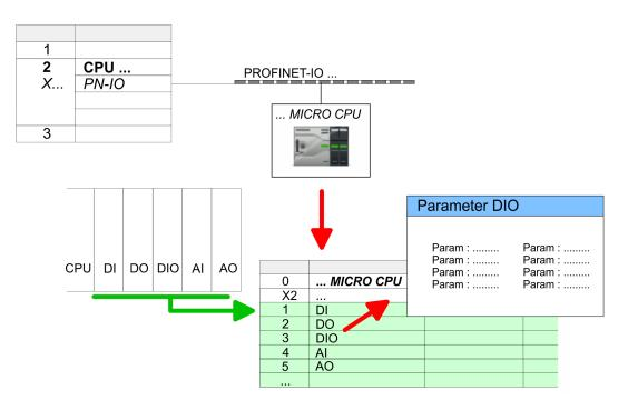
Hardware configuration - Ethernet PG/OP channel
