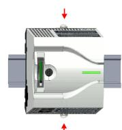
To fix the CPU at the mounting rail, move the locking levers back to the initial posi-6. tion.
