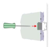
**1.** Remove the bus cover with a screwdriver on the right side of the CPU.
