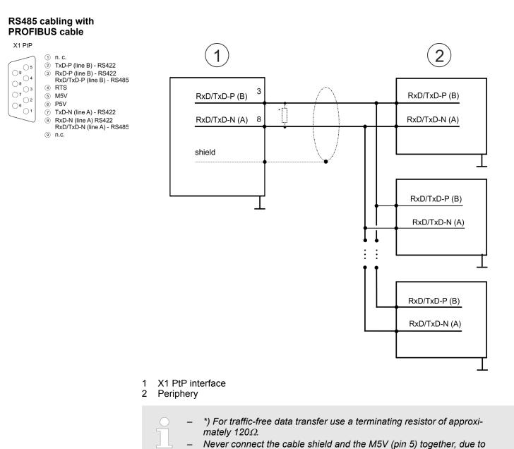
the compensation currents the interfaces could be destroyed!
