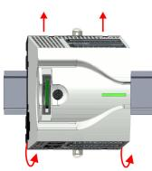
**2.** Remove the CPU with a rotation upwards from the mounting rail.
