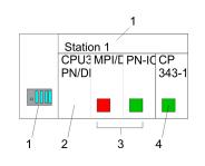
1 *Station:* This includes a PLC station with rack, CPU and communication components. Via the context menu you may configure a station added from the net objects and its
