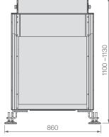
This operating platform enables the mounting of HC10-series robots in ergonomic height and provides space for the robot cable and the control MOTOMAN YRC1000. Due to the weight of 114 kg, the platform can be relocated easily with a hand pallet truck.
