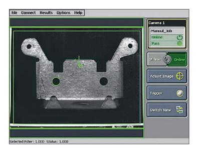
The MotoSight2D Vision combines leading vision technology with leading robotic technology. The MotoSight2D product range is based on compact 2D cameras in 3 different performance classes. In addition to simple data exchange, programming of the camera from the teach pendant of the robot is also possible.
