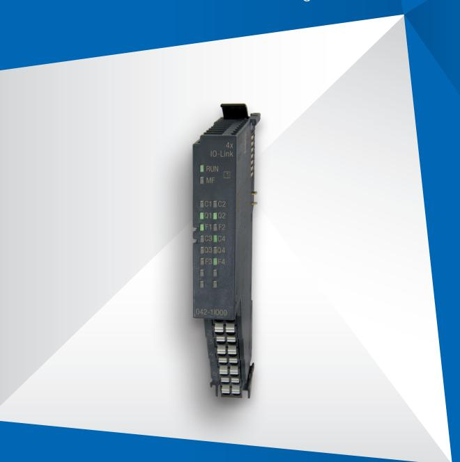
The proven decentralized I/O and control system SLIO is now extended by a new IO-Link module and the associated software YASKAWA IO-Link Manager. The SLIO IO-Link module now enables communication between CPU and IO-Link capable field devices such as sensors and actuators according to IEC 61131-9.
