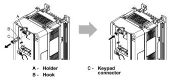
Figure 5.5 Moving the Keypad Connector to the Holder
