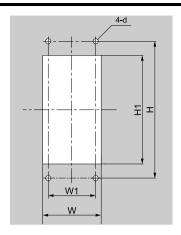
Figure 5.7 Internal/Flush-Mount Enclosure Panel Cut-Out Dimensions
