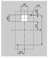
Figure 5.13 External/Face Mount Enclosure Panel Cut-Out
