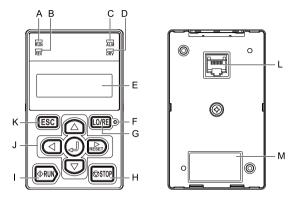
Figure 4.1 Keypad Components
