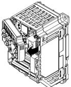
Figure 5.24 Removing the Included Drive Keypad
