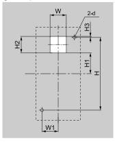
Figure 5.2 External/Face Mount Enclosure Panel Cut-Out Dimensions
