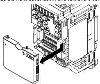
Figure 5.16 Remove the Front Cover
