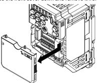
Figure 5.23 Remove the Front Cover
