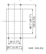
Figure 10 Panel Cut-out Dimensions (Internal/Flush-mount Installation)
