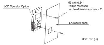
Figure 7 External/Face-mount Installation
