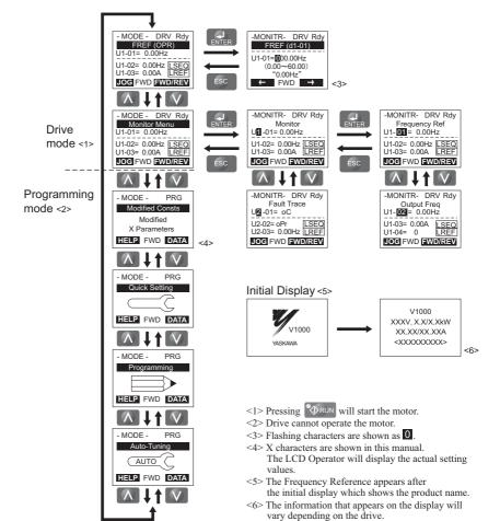
Figure 12 LCD Operator Option Menu Structure
