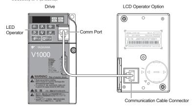
Figure 11 Communication Cable Connection
