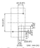
Figure 8 Panel Cut-out Dimensions (External/Face-mount Installation)
