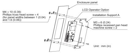
Figure 9 Internal/Flush Mount Installation
